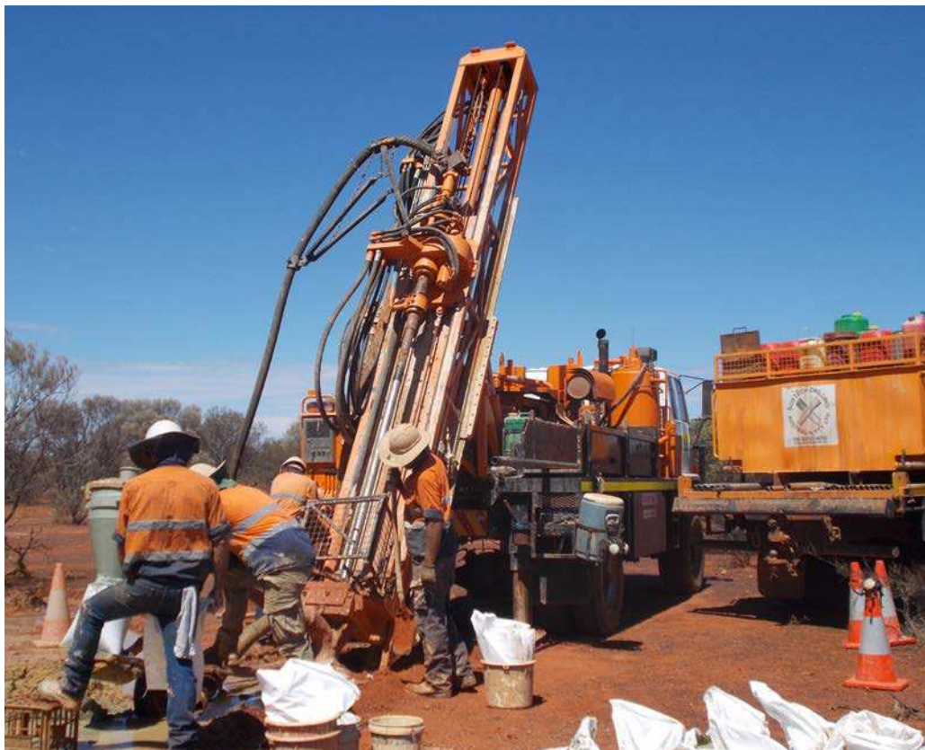
Plate 2: AC/RC Drill Rig at Indomitabile
