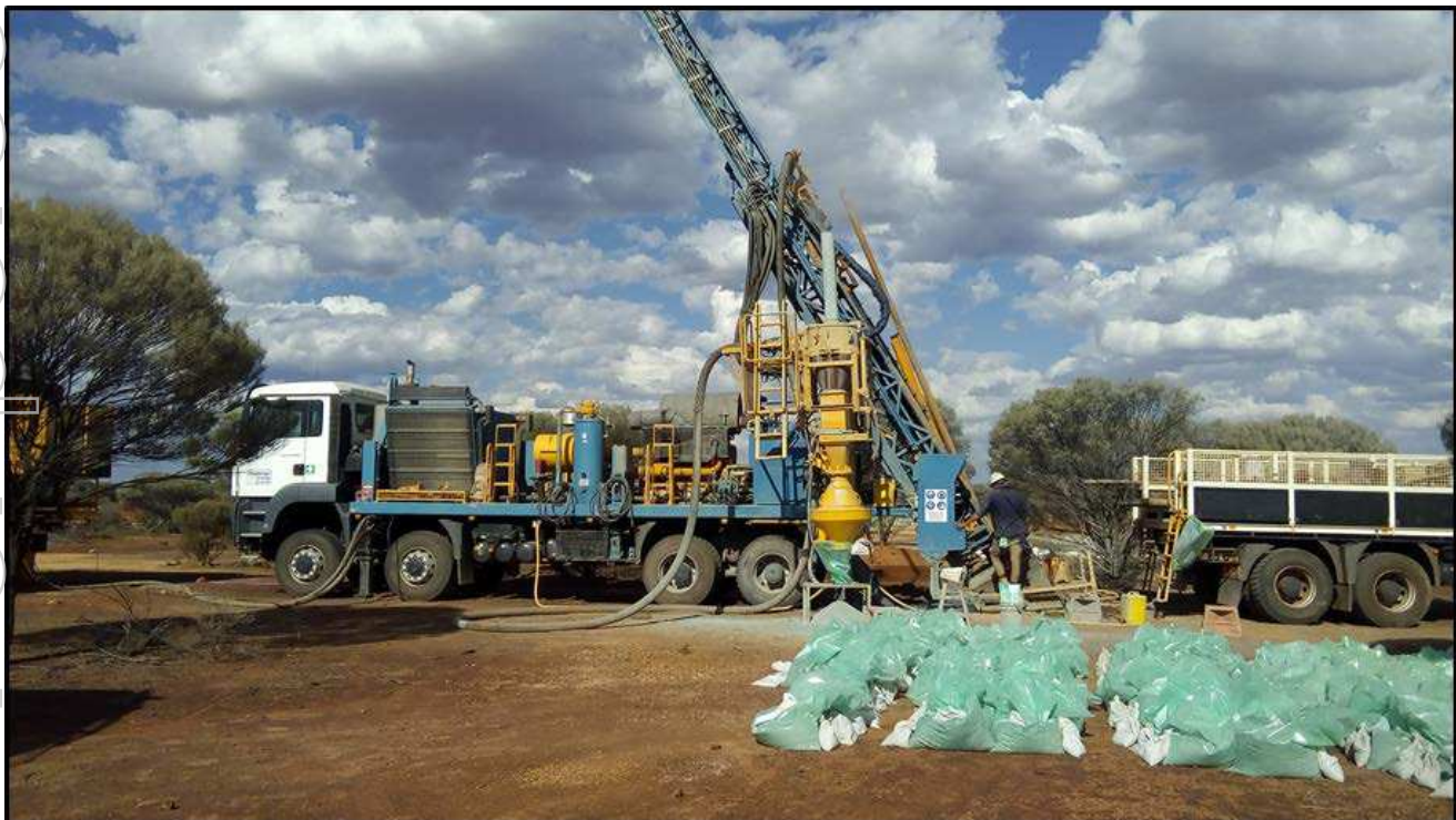
Plate 1. RC drilling (Hole SRC 036) at Vanguard, October 2017
